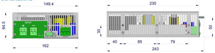
Lateral fixing holes 6 x M4 (screw torque < 1.6 Nm). Maximum screw deep 6 mm.
