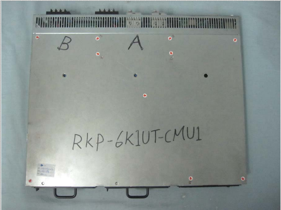
View of Discharge Point-5 (Red: Contact discharge)
