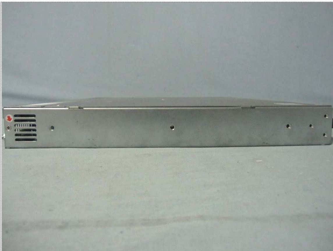
View of Discharge Point-3 (Red: Contact discharge)
